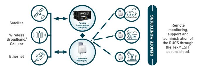
DMs extend network signal from a PCL or any Ethernet source. They broadcast signal locally over a 1000+ ft radius and extend signal over a wide area through a wireless mesh network.
